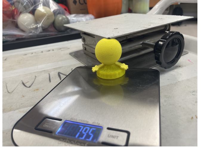
FIG. 2. Setup for the mechanical work portion of the experiment showing digital scale, popper, and scissor jack. Popper is shown at onset of snap-through instability.
